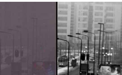
Extreme fog conditions - Left: Visible, Right - SWIR
