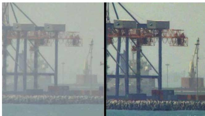
Digital stabilization and image enhancement (Left: OFF, Right:ON)
